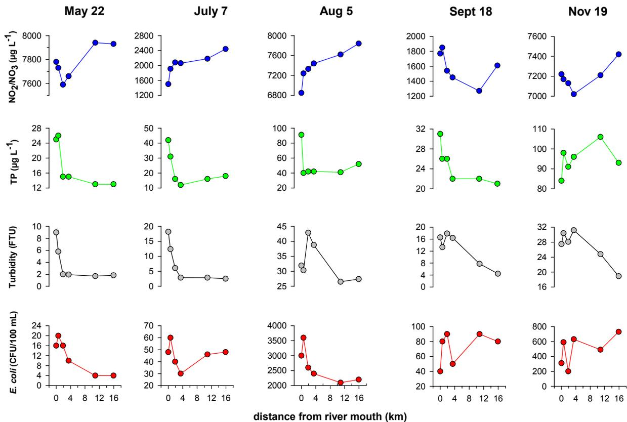
Figure 10: Water quality measures at stations ranging from the intensive monitoring station to the mouth of the Bayfield River on each of the nearshore survey dates.
