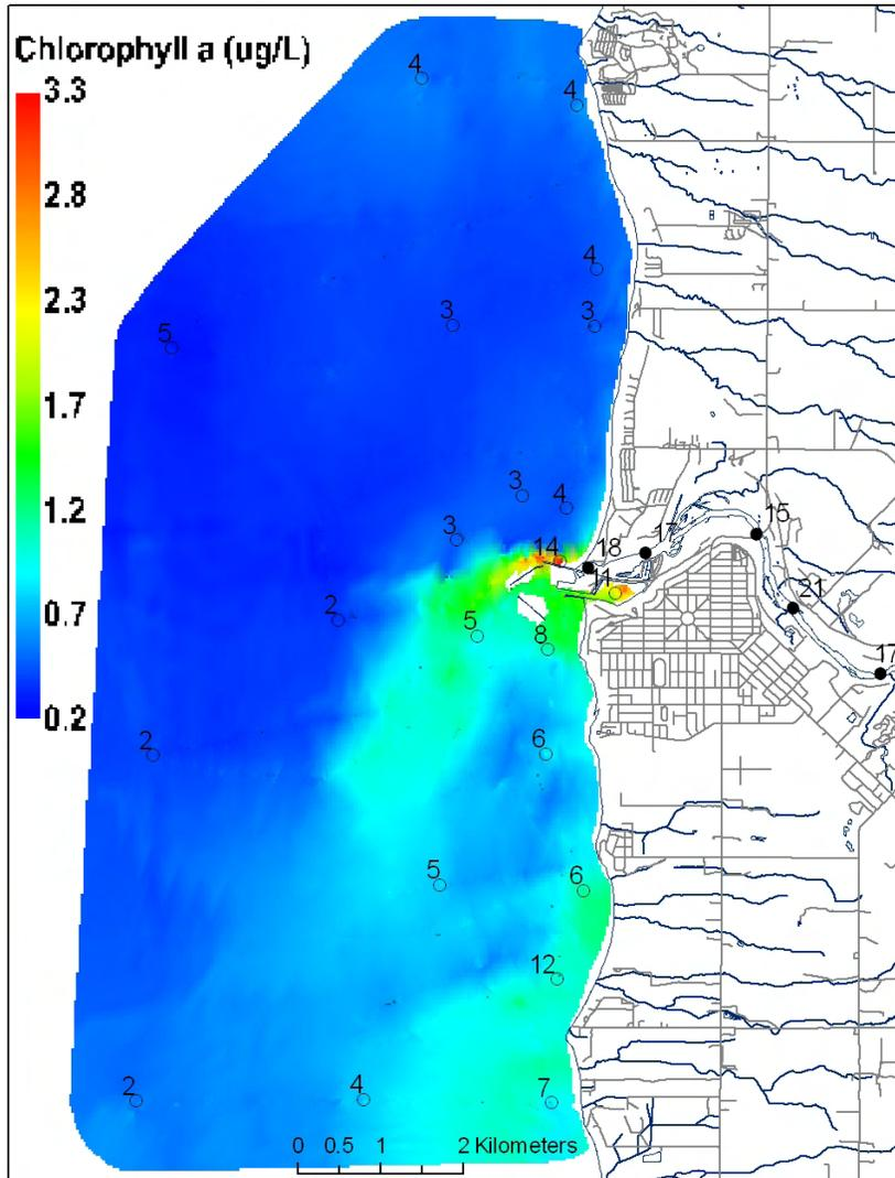
Figure 25: Surface chl a concentration estimated from fluorescence (colour scale;  $\mu\text{g L}^{-1}$ ) and TP concentrations (point samples;  $\mu\text{g L}^{-1}\text{P}$ ) at the Maitland River study area during the spring survey (May 27, 2003).
