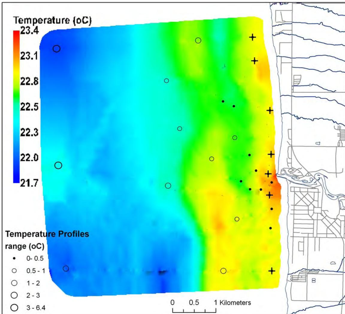
Figure 42: Surface water temperature (°C) at the Bayfield River Survey area during the late summer survey (August 5, 2003). The crosses indicate locations where water column was well mixed using a criterion of  $< 0.01 \text{ g cm}^{-3}$  change per meter drop.
