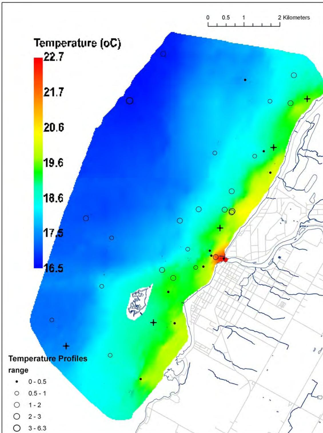
Figure 32: Surface water temperature (°C) at the Saugeen River study area during the second summer survey (July 29, 2003). The circles indicate locations of depth profiles of temperature with size proportional to temperature change with depth. The crosses indicate locations where water column was well mixed using a criterion of  $< 0.01 \text{ g cm}^{-1}$  change per meter drop.
