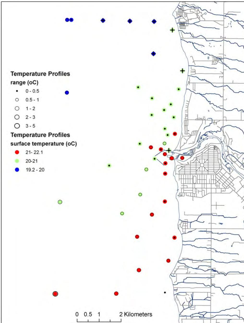
Figure 37: Surface water temperature (°C) at the Maitland River study area during the second summer survey (July 31, 2003). The circles indicate locations of depth profiles of temperature with size proportional to temperature change with depth. The crosses indicate locations where water column was well mixed using a criterion of  $< 0.01 \text{ g cm}^{-1}$  change per meter drop.
