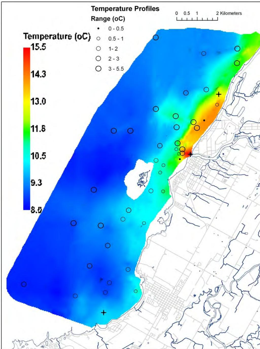
Figure 27: Surface water temperature (°C) at the Saugeen River study area during the spring survey (May 28, 2003). The circles indicate locations of depth profiles of temperature with size proportional to temperature change with depth. The crosses indicate locations where water column was well mixed using a criterion of  $< 0.01 \text{ g cm}^{-3}$  change per meter drop.
