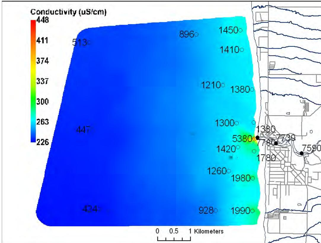
Figure 18: Surface conductivity (colour scale;  $\mu\text{S cm}^{-1}$  at  $25^\circ\text{C}$ ) and  $\text{NO}_2+\text{NO}_3$  concentrations (point samples;  $\mu\text{g L}^{-1} \text{N}$ ) at the Bayfield River study area during the spring survey (May 22, 2003).
