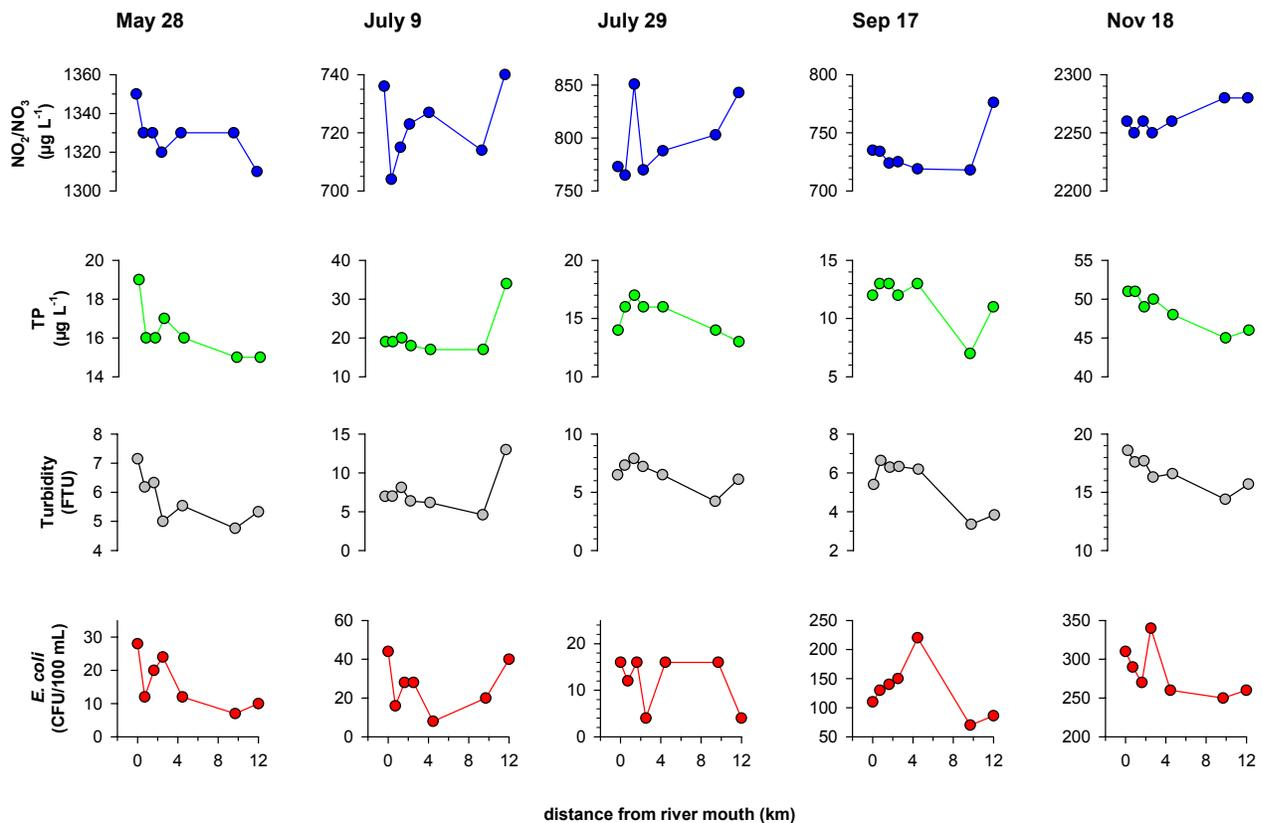
Figure 8: Water quality measures at stations extending from the intensive monitoring station to the mouth of the Saugeen River on each of the nearshore survey dates (see Table 2).
