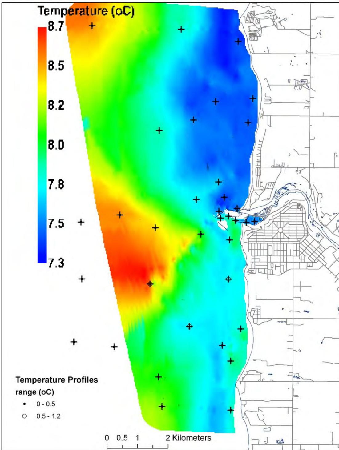
Figure 57: Surface water temperature ( $^{\circ}\text{C}$ ) at the Maitland River survey area during the second fall survey (November 23, 2003). The crosses indicate locations where water column was well mixed using a criterion of  $< 0.01 \text{ g cm}^{-3}$  change per meter drop.
