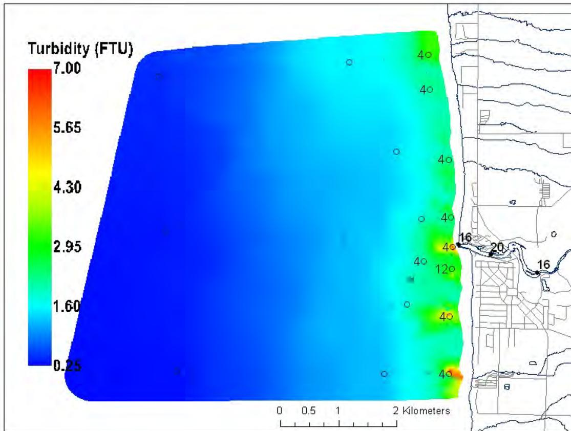
Figure 19: Surface turbidity (colour scale; FTU) and *E. coli* concentrations (point samples; CFU 100 mL<sup>-1</sup>) at the Bayfield River study area during the spring survey (May 22, 2003). No samples were collected at points without numeric values.
