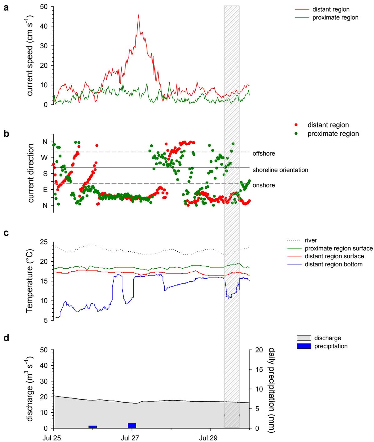
Figure 31: Saugeen River study area second summer survey (July 29, 2003). Physical conditions in the days before and during the survey (hatched region). Current speed (**a**) and direction (**b**) in the distant and proximate regions, temperature of the Saugeen River and the distant and proximate regions (**c**), Saugeen River discharge and local precipitation (**d**).
