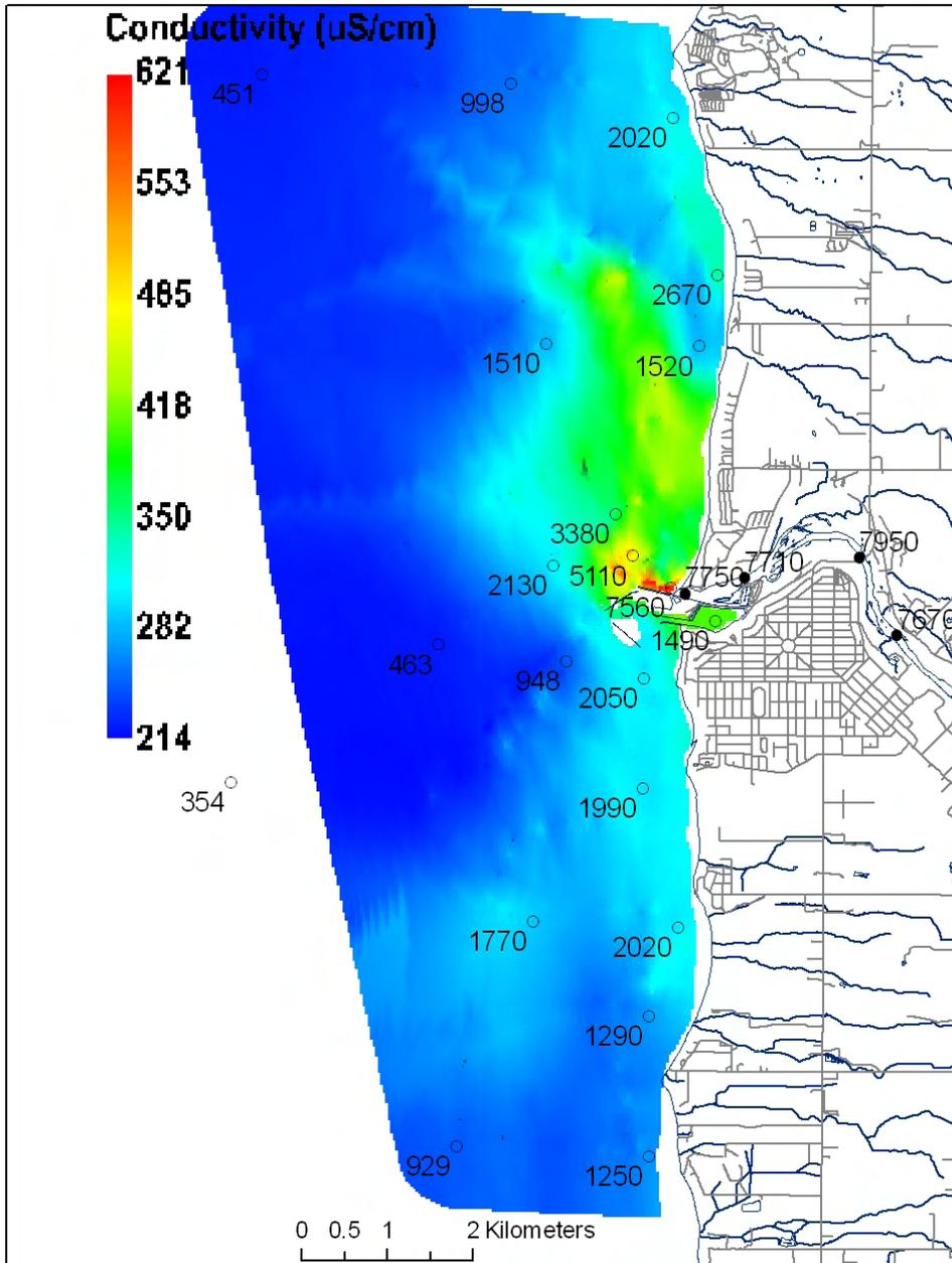
Figure 58: Surface conductivity (colour scale;  $\mu\text{S cm}^{-1}$  at 25°C) and NO<sub>2</sub>+NO<sub>3</sub> concentrations (point samples;  $\mu\text{g L}^{-1}$  N) at the Maitland River study area during the second fall survey (November 23, 2003).
