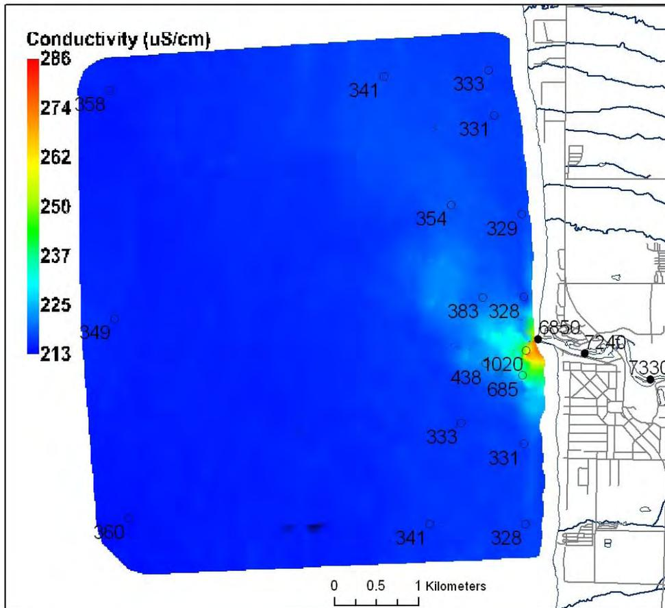
Figure 43: Surface conductivity (colour scale;  $\mu\text{S cm}^{-1}$  at 25°C) and  $\text{NO}_2+\text{NO}_3$  concentrations (point samples;  $\mu\text{g L}^{-1}\text{N}$ ) at the Bayfield River study area during the second summer survey (August 5, 2003).
