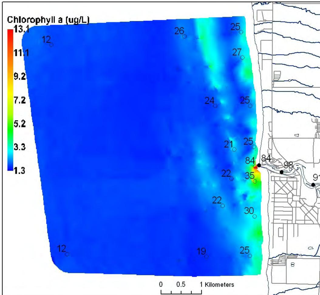
Figure 55: Surface chlorophyll *a* estimated from fluorescence (colour scale;  $\mu\text{g L}^{-1}$ ) and TP concentrations (point samples;  $\mu\text{g L}^{-1}$  P) at the Bayfield River study area during the second fall survey (November 19, 2003).
