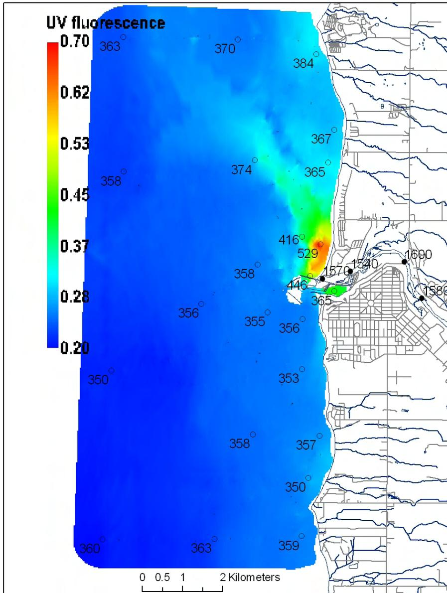
Figure 38: Surface UV fluorescence (colour scale; relative to  $\mu\text{g L}$  of compound carbazole) and  $\text{NO}_2+\text{NO}_3$  concentrations (point samples;  $\mu\text{g L}^{-1}\text{N}$ ) at the Maitland River study area during the second summer survey (July 31, 2003).
