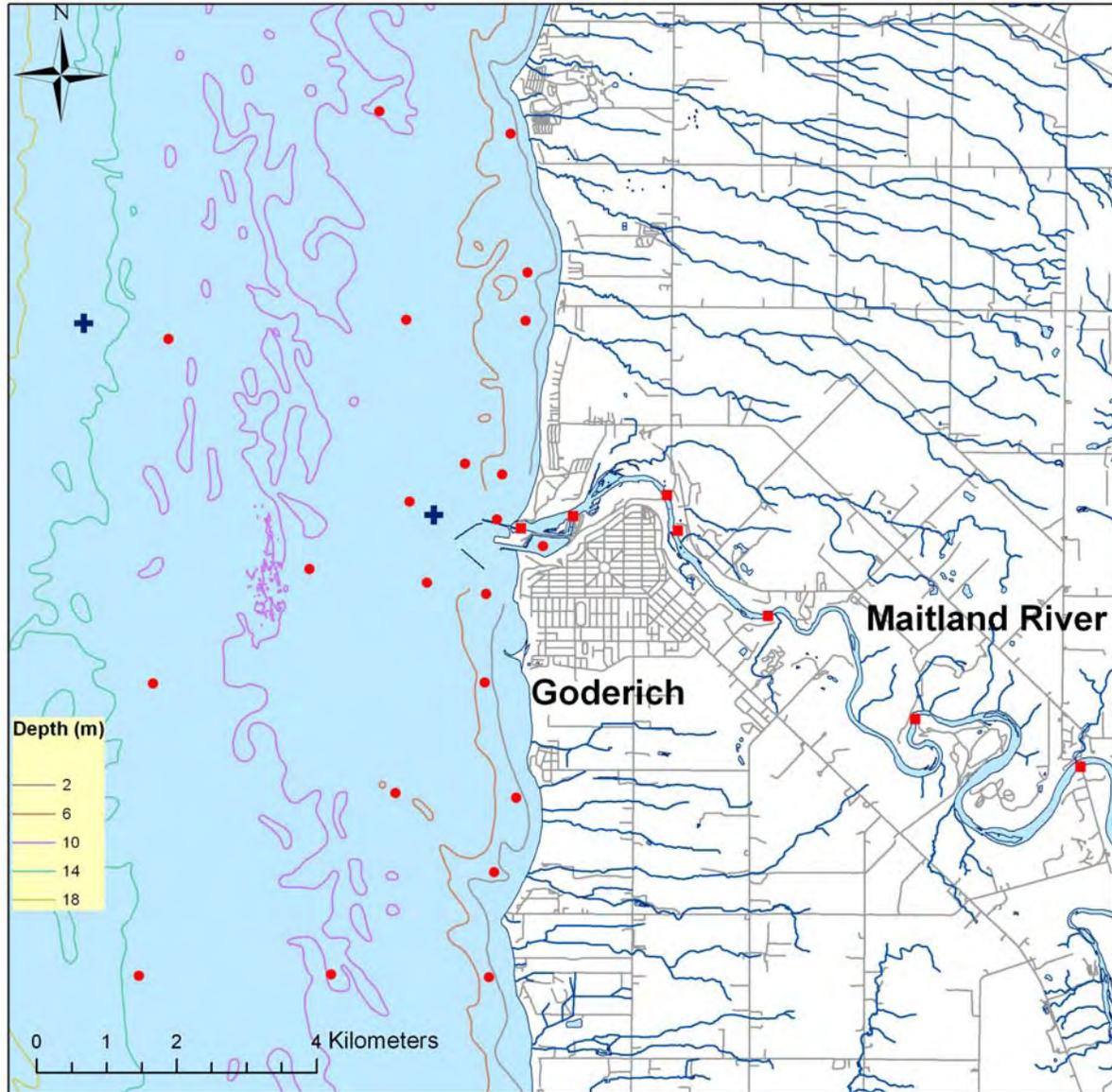
Figure 3: Map of the Maitland River study area showing locations of discrete sampling stations (●) in the nearshore and river. Positions of instrumentation (temperature recorders and current meters) deployed over the study periods (+) are also shown.
