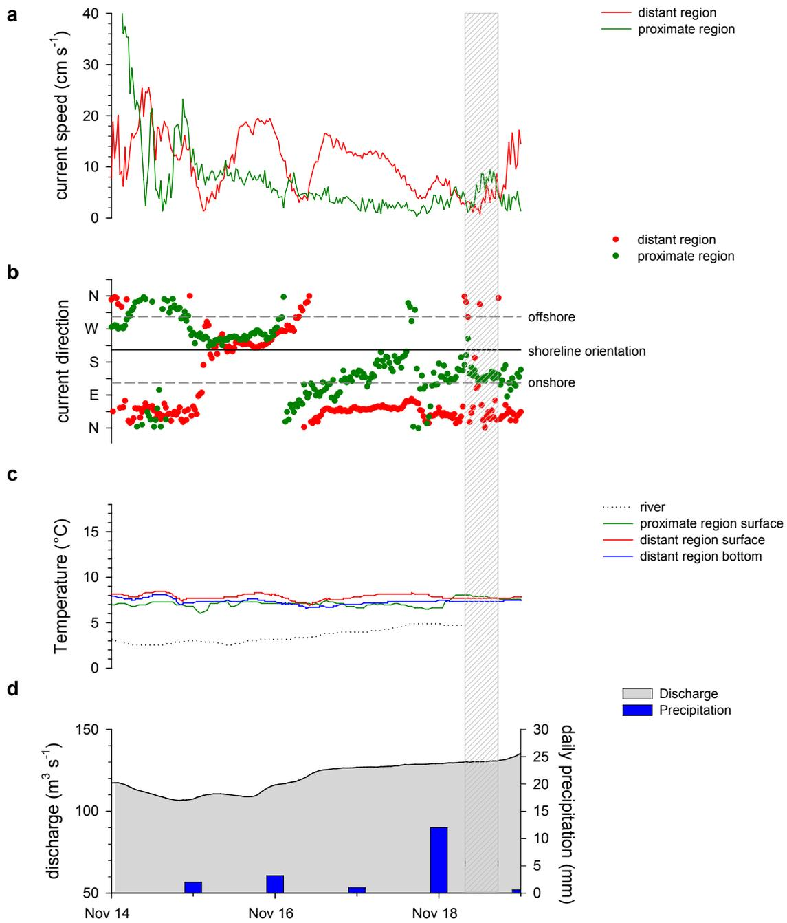
Figure 46: Saugeen Fall 2 survey. Physical conditions in the days before and during the survey (hatched region). Current speed (**a**) and direction (**b**) in the distant and proximate regions, temperature of the Saugeen River and the distant and proximate regions (**c**), Saugeen River discharge and local precipitation (**d**). See sections 2.3 and 2.5 for details.
