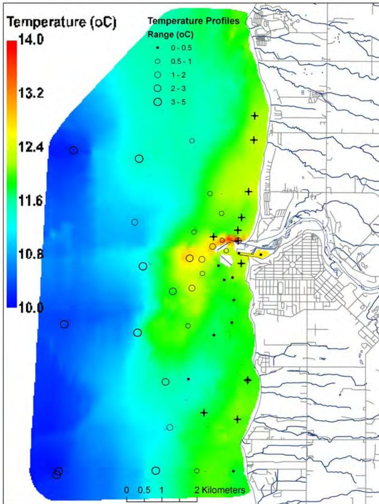
Figure 22: Surface water temperature ( $^{\circ}\text{C}$ ) at the Maitland River study area during the spring summer survey (May 27, 2003). The circles indicate locations of depth profiles of temperature with size proportional to temperature change with depth. The crosses indicate locations where water column was well mixed using a criterion of  $< 0.01 \text{ g cm}^{-3}$  change per meter drop.
