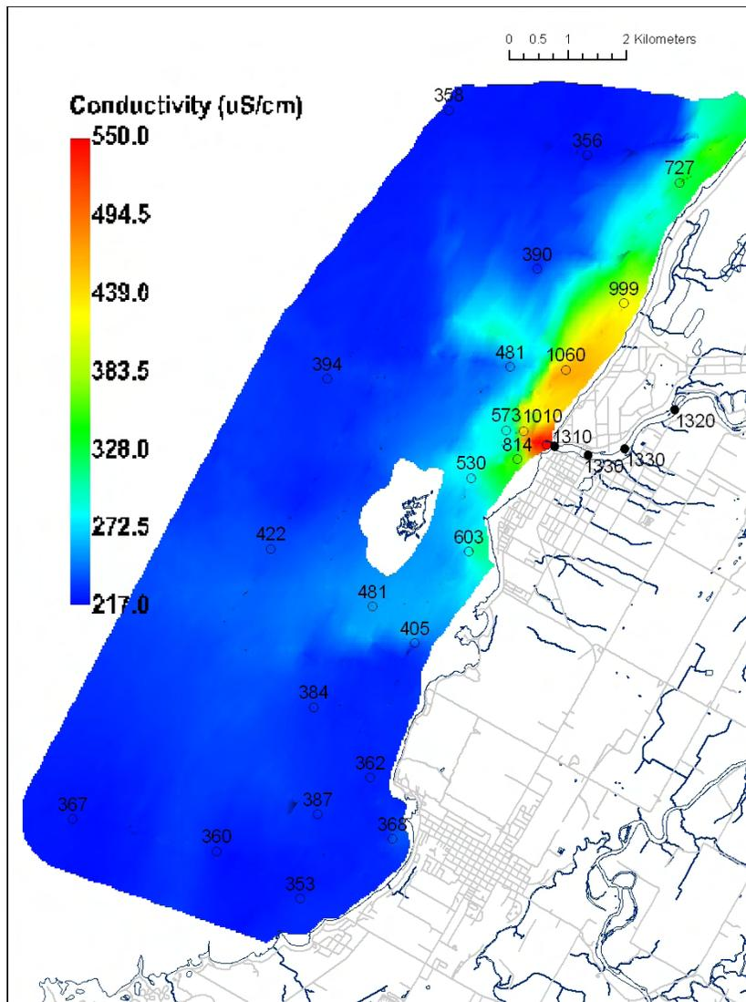
Figure 28: Surface conductivity (colour scale;  $\mu\text{S cm}^{-1}$  at  $25^\circ\text{C}$ ) and  $\text{NO}_2+\text{NO}_3$  concentrations (point samples;  $\mu\text{g L}^{-1}\text{N}$ ) at the Saugeen River study area during the spring survey (May 28, 2003).
