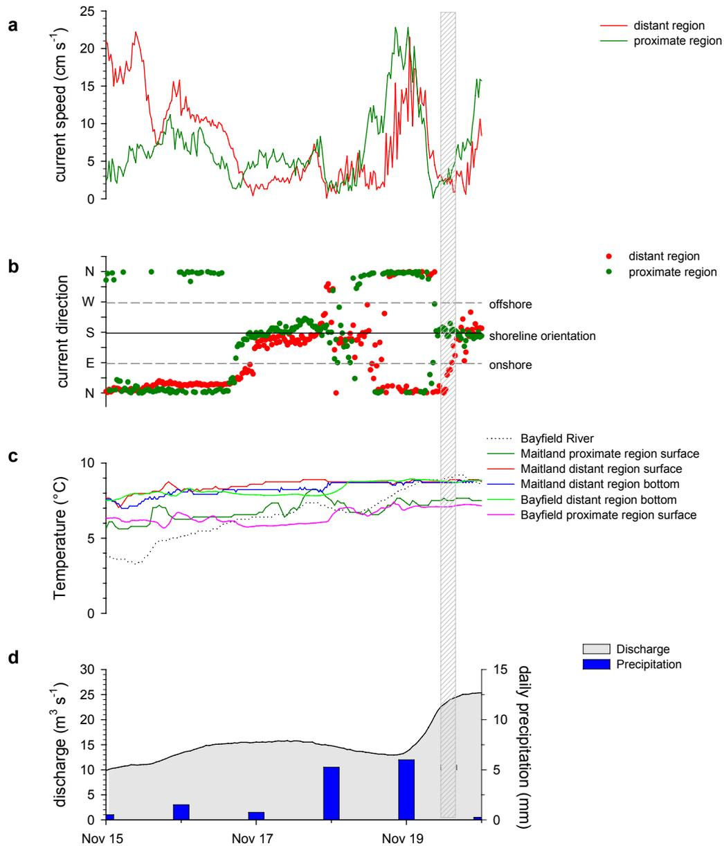
Figure 51: Bayfield second fall survey (November 19, 2003). Physical conditions in the days before and during the survey (hatched region). Current speed (**a**) and direction (**b**) in the distant and proximate regions, temperature of the Bayfield River and the distant and proximate regions (note that some data are for the Maitland study area) (**c**), Bayfield River discharge and local precipitation (**d**). See sections 2.3 and 2.5 for details.
