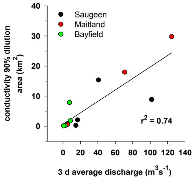
Figure 15: Linear regression between river plume size (conductivity 90% dilution area) and 3-day average river discharge across all rivers and survey dates (for which data were available)
