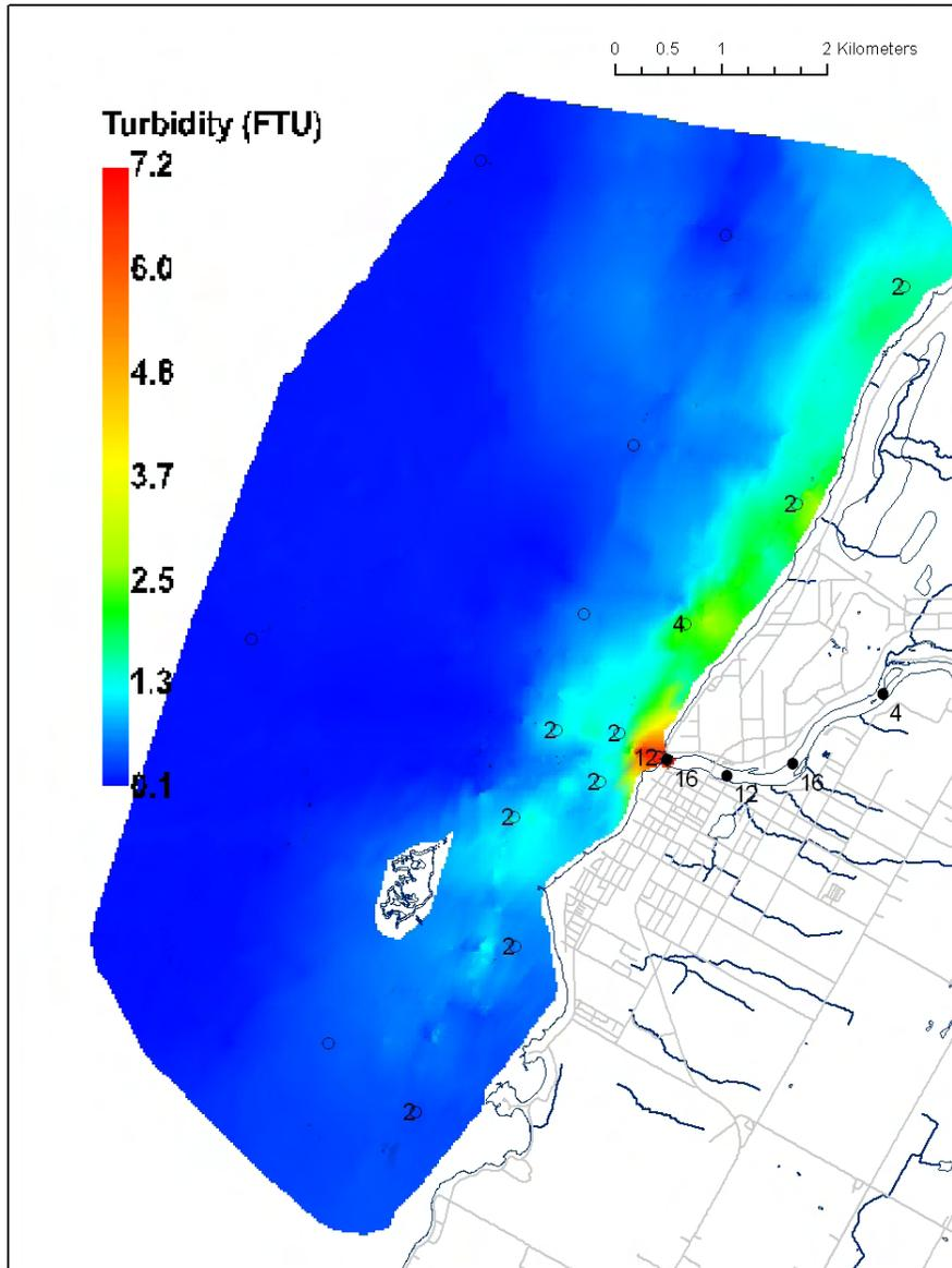
Figure 34: Surface turbidity (colour scale; FTU) and *E. coli* concentrations (point samples; CFU 100 mL<sup>-1</sup>) at the Saugeen River study area during the second summer survey (July 29, 2003). No samples were collected at points without numeric values.
