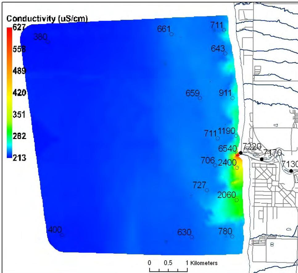
Figure 53: Surface conductivity (colour scale;  $\mu\text{S cm}^{-1}$  at  $25^\circ\text{C}$ ) and  $\text{NO}_2+\text{NO}_3$  concentrations (point samples;  $\mu\text{g L}^{-1} \text{N}$ ) at the Bayfield River study area during the second fall survey (November 19, 2003).
