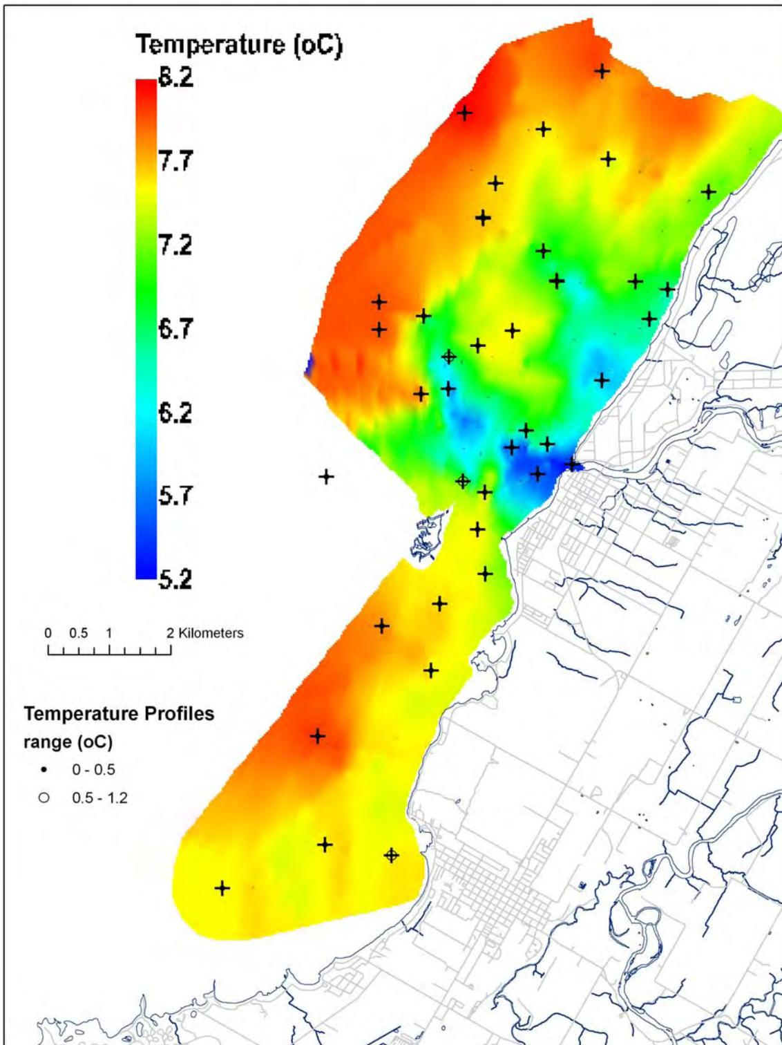
Figure 47: Surface water temperature ( $^{\circ}\text{C}$ ) at the Saugeen River study area during the second fall survey (November 18, 2003). The crosses indicate locations where water column was well mixed using a criterion of  $< 0.01 \text{ g cm}^{-3}$  change per meter drop.
