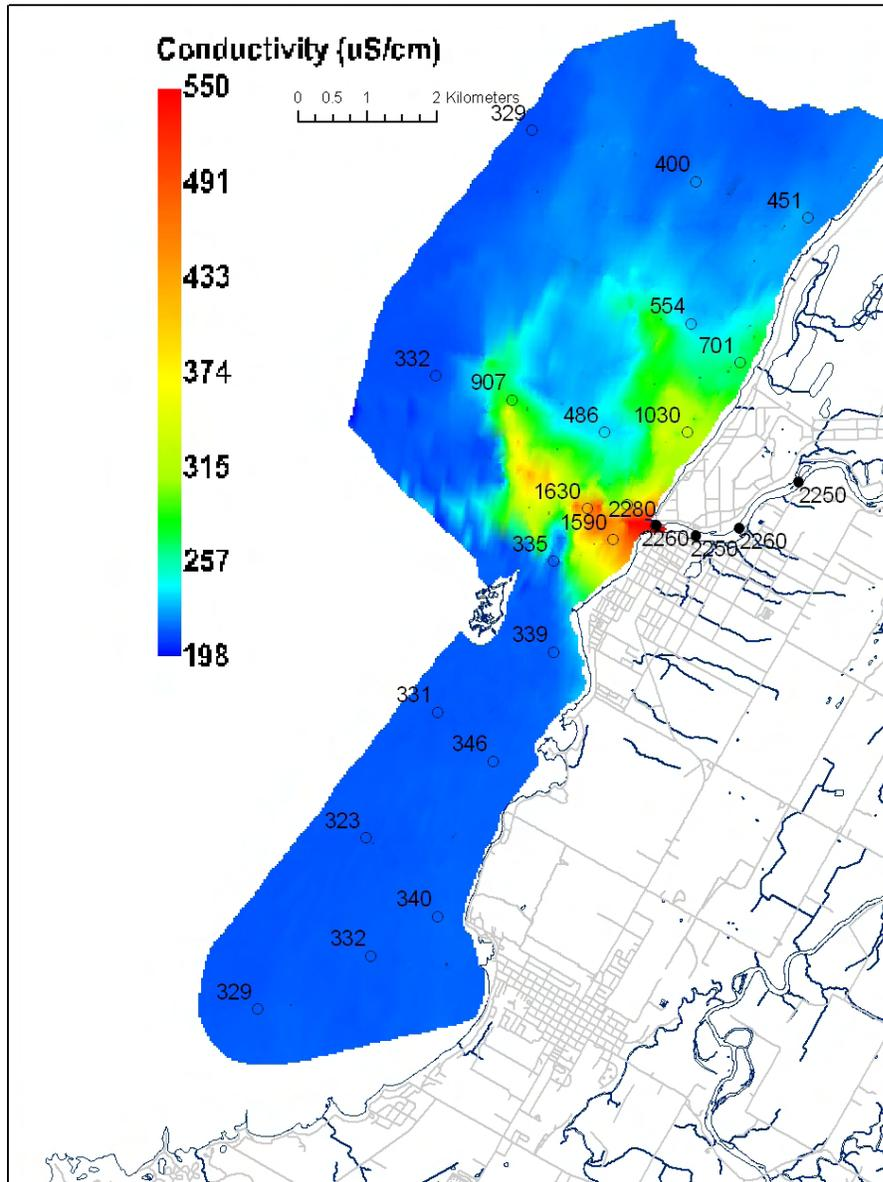
Figure 48: Surface conductivity (colour scale;  $\mu\text{S cm}^{-1}$  at  $25^\circ\text{C}$ ) and  $\text{NO}_2+\text{NO}_3$  concentrations (point samples;  $\mu\text{g L}^{-1} \text{N}$ ) at the Saugeen River study area during the second fall survey (November 18, 2003).
