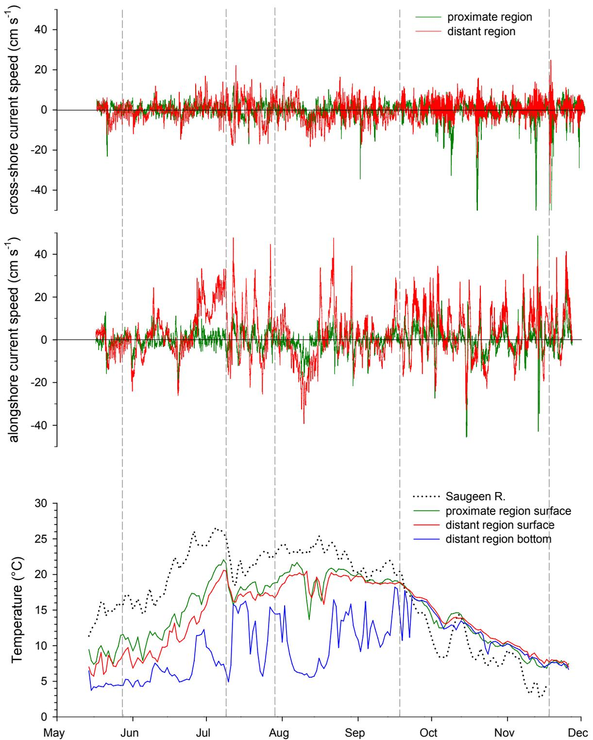
Figure 11: Cross-shore and alongshore current speeds and daily mean water temperature in the proximate and distant regions of the Saugeen River study area and at the mouth of the river in 2003. Positive cross-shore and alongshore current speeds are East and North-directed currents, respectively. See Figure 2 for locations of instrumentation. Current speeds are for the water layer approximately 3 to 5 m from surface. Dashed vertical lines indicate the time of nearshore water quality surveys.
