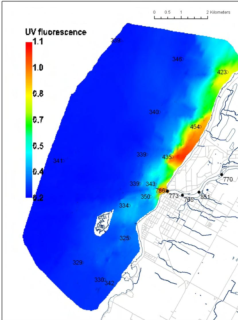
Figure 33: Surface UV fluorescence (colour scale; relative to  $\mu\text{g L}^{-1}$  of compound carbazole) and  $\text{NO}_2+\text{NO}_3$  concentrations (point samples;  $\mu\text{g L}^{-1}\text{N}$ ) at the Saugeen River study area during the second summer survey (July 29, 2003).
