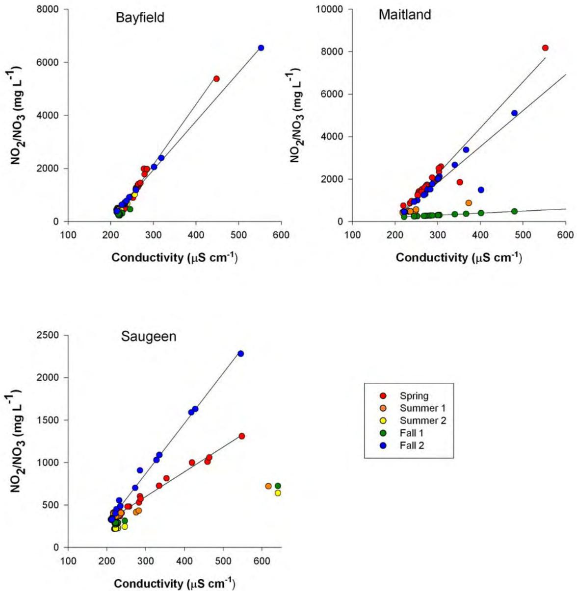
Figure 14: Linear regressions between  $\text{NO}_2+\text{NO}_3$  concentration and field conductivity at the survey area. Field conductivity has been adjusted using survey-specific regressions of field against lab-measured conductivity to minimize the effects of variance in calibration of the field sensor over surveys and among study areas.
