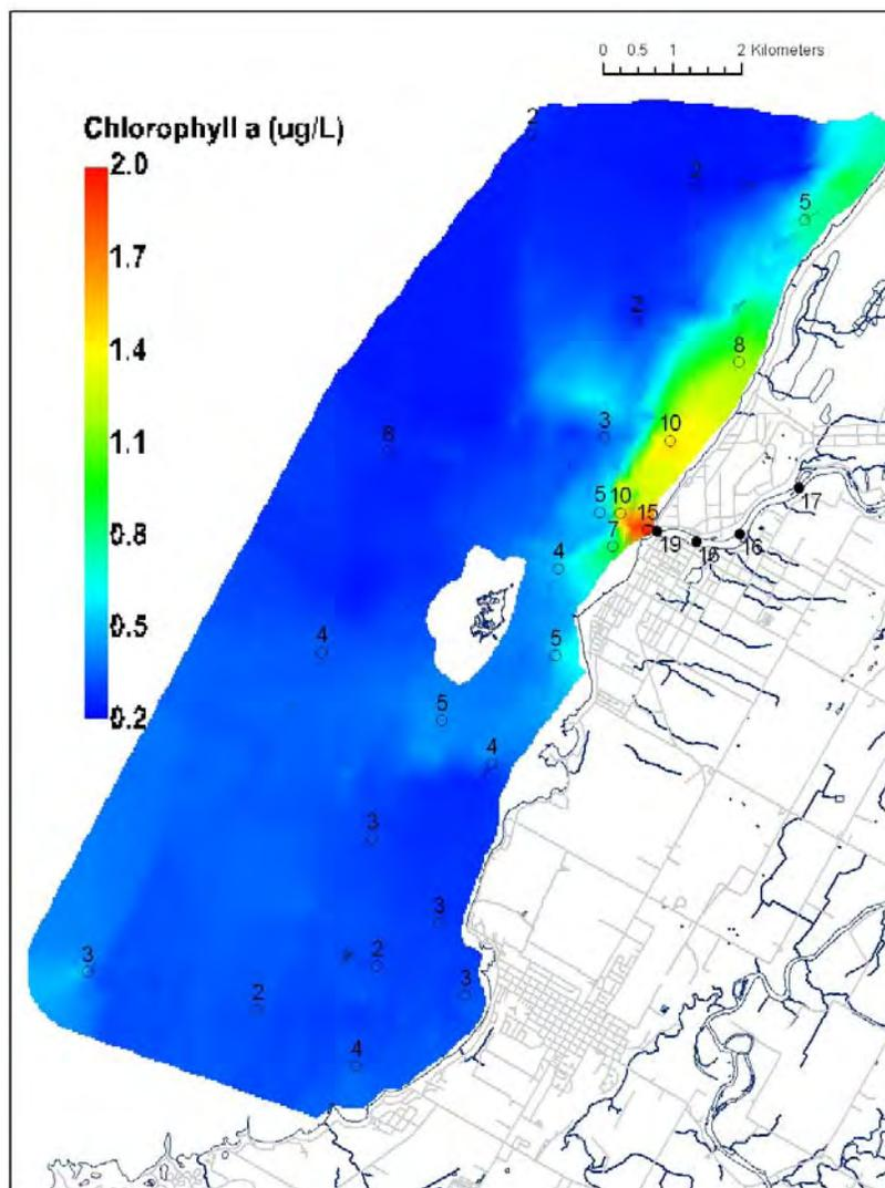
Figure 30: Surface chlorophyll a estimated from fluorescence (colour scale;  $\mu\text{g L}^{-1}$ ) and TP concentrations (point samples;  $\mu\text{g L}^{-1}$  P) at the Saugeen River study area during the spring survey (May 28, 2003).
