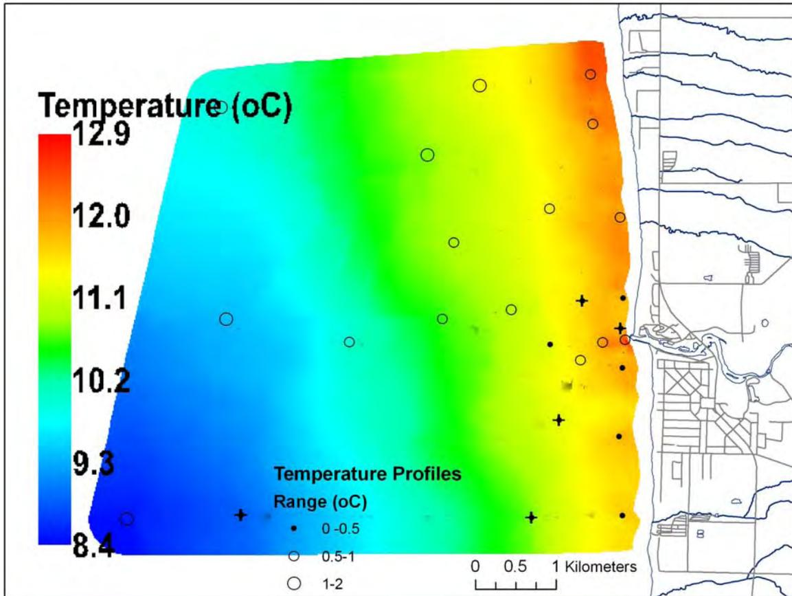
Figure 17: Surface water temperature ( $^{\circ}\text{C}$ ) at the Bayfield River survey area during the spring survey (May 22, 2003). The circles indicate locations of depth profiles of temperature with size proportional to temperature change with depth. The crosses indicate locations where water column was well mixed using a criterion of  $< 0.01 \text{ g cm}^{-3}$  (density) change per meter drop.
