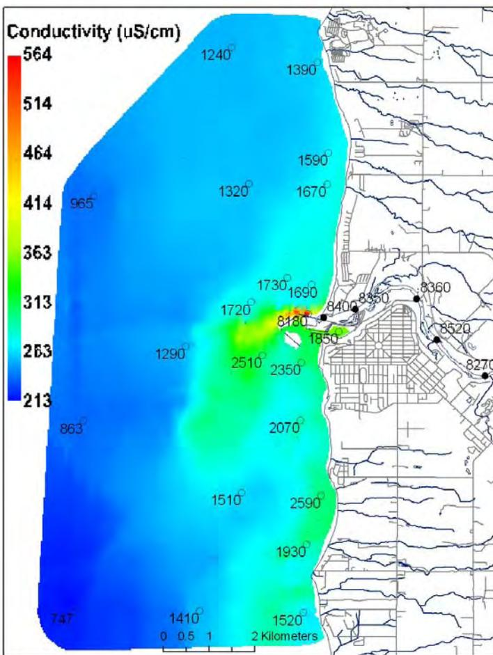
Figure 23: Surface conductivity (colour scale;  $\mu\text{S cm}^{-1}$  at  $25^\circ\text{C}$ ) and  $\text{NO}_2 + \text{NO}_3$  concentrations (point samples;  $\mu\text{g L}^{-1} \text{N}$ ) at the Maitland River study area during the spring survey (May 27, 2003).
