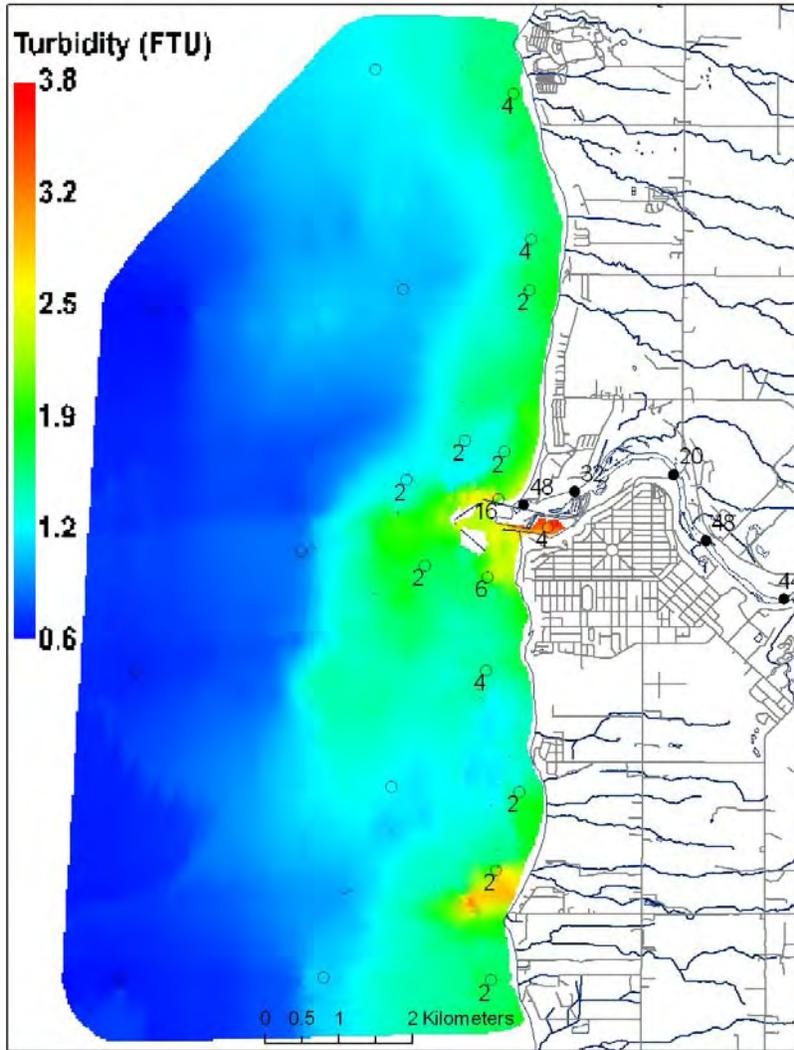
Figure 24: Surface turbidity (colour scale; FTU) and *E. coli* concentrations (point samples; CFU 100 mL<sup>-1</sup>) at the Maitland River study area during the spring survey (May 27, 2003). Samples were not collected at points without numeric values.
