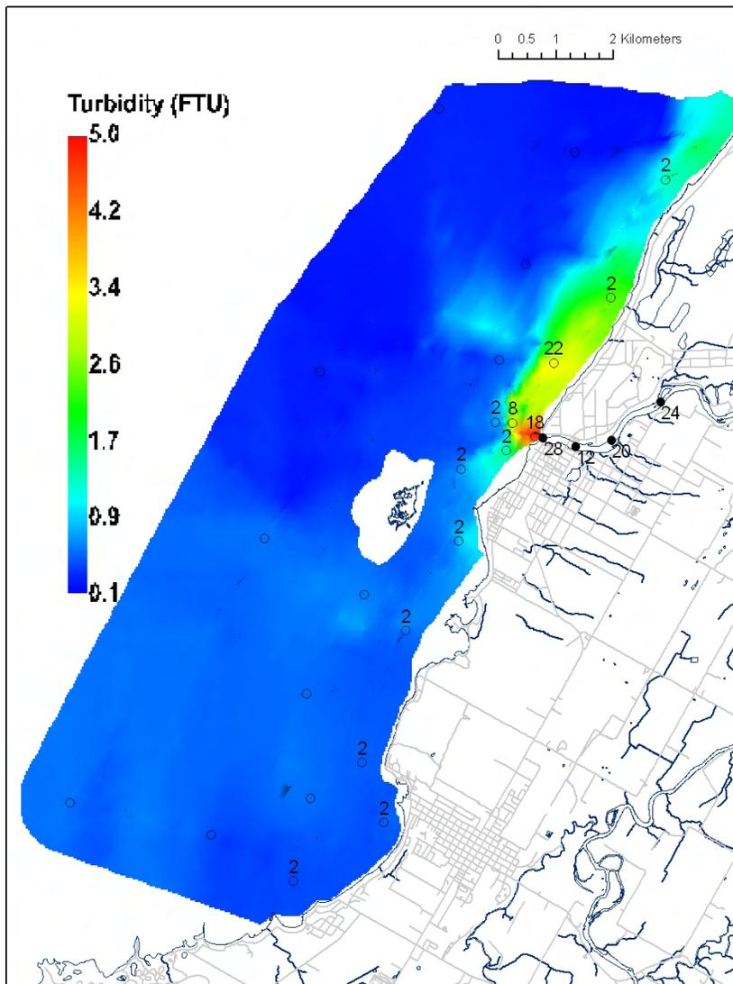
Figure 29: Surface turbidity (colour scale; FTU) and *E. coli* concentrations (point samples; CFU 100 mL<sup>-1</sup>) at the Saugeen River study area during the spring survey (May 28, 2003). No samples collected at points without numeric values.
