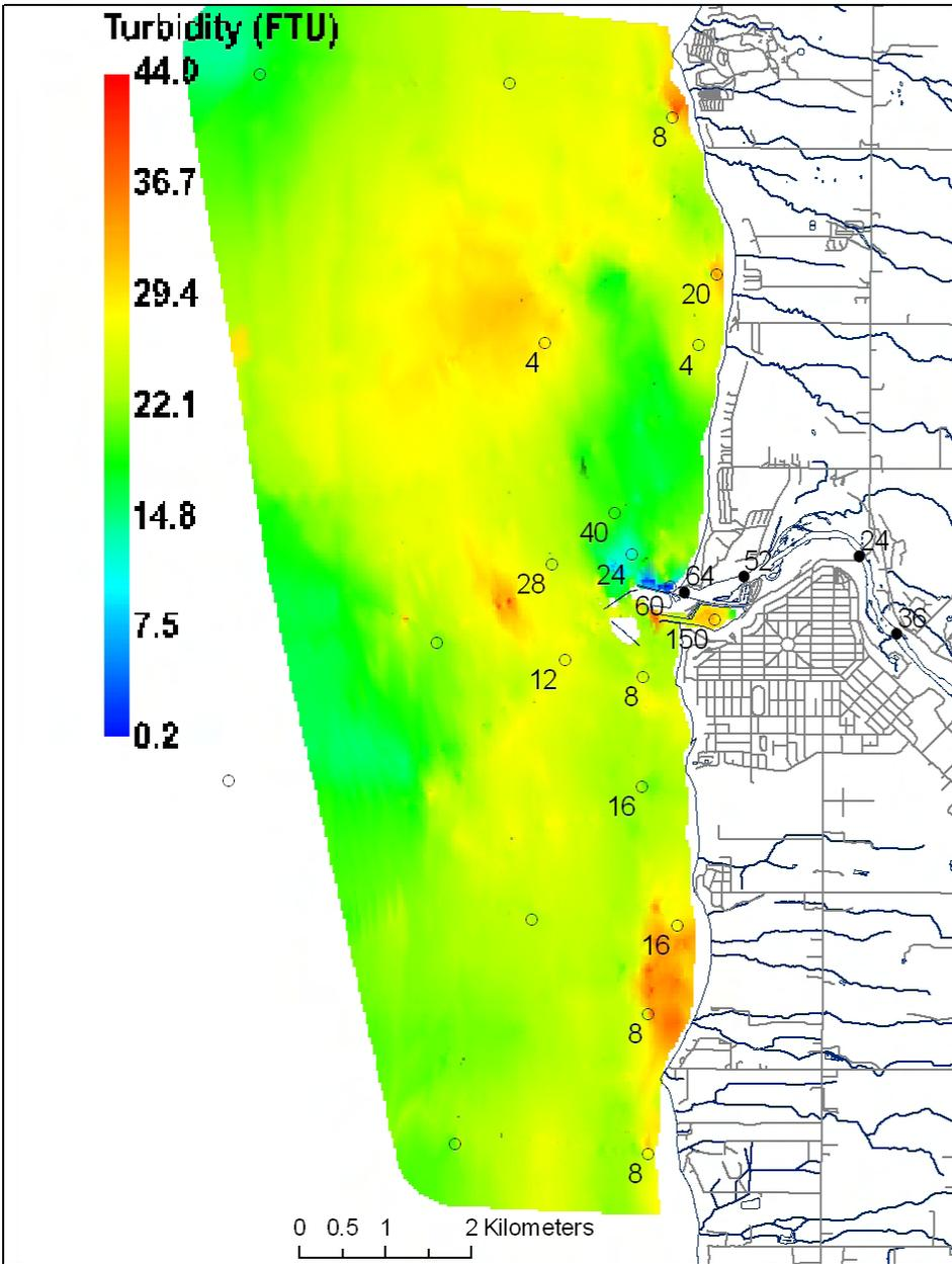
Figure 59: Surface turbidity (colour scale; FTU) and *E. coli* concentrations (point samples; CFU 100 mL<sup>-1</sup>) at the Maitland River study area during the second fall survey (November 23, 2003). No samples were collected at points without numeric values.
