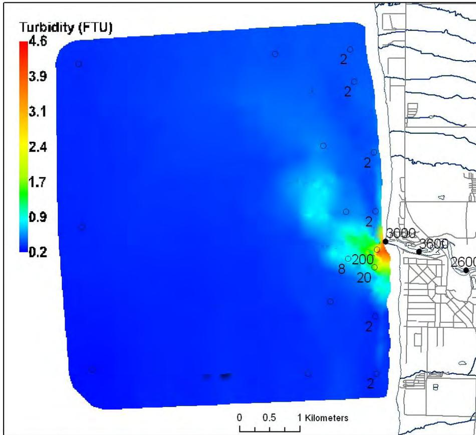
Figure 44: Surface turbidity (colour scale; FTU) and *E. coli* concentrations (point samples; CFU 100 mL<sup>-1</sup>) at the Bayfield River study area during the second summer survey (August 5, 2003). No samples were collected at points without numeric values.
